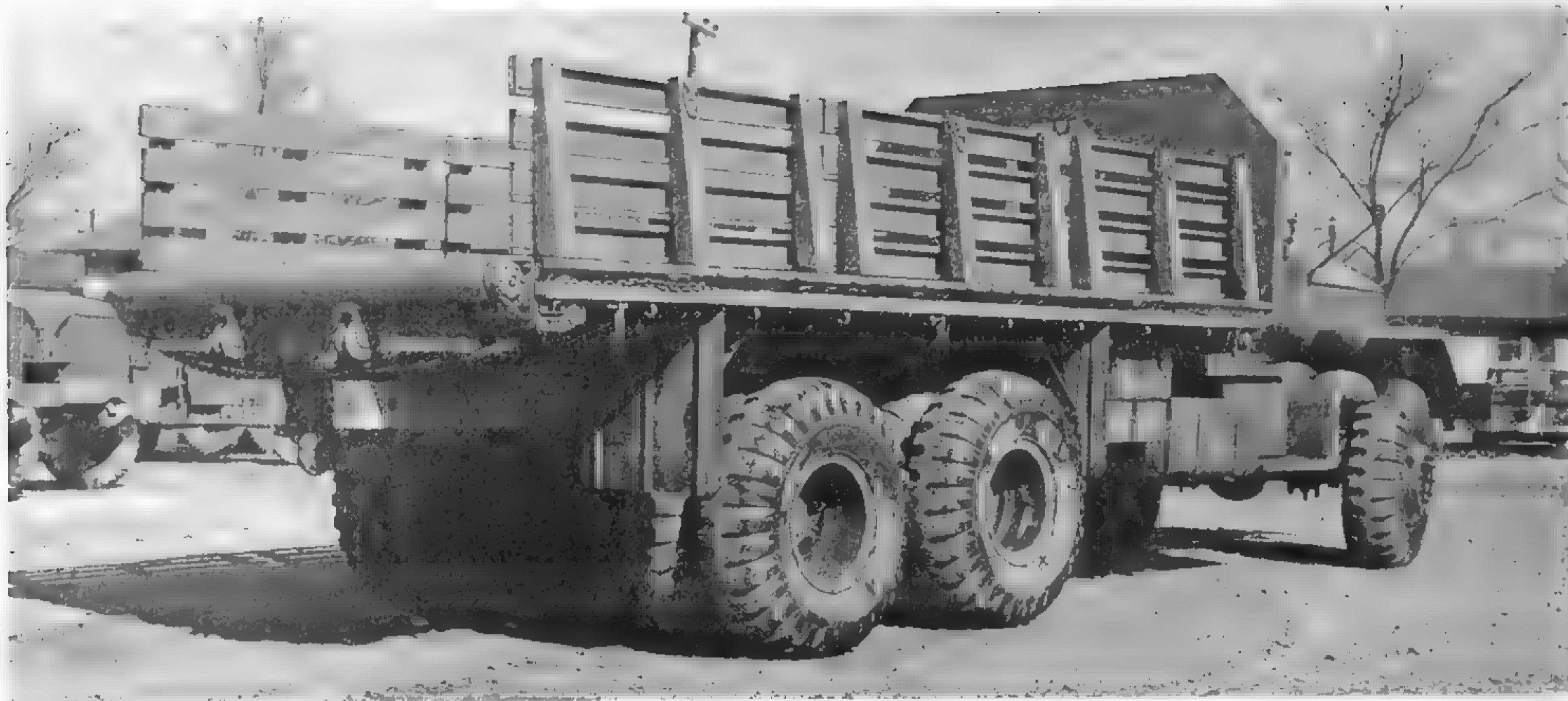
At the rear of the large all-steel bed on the M328 was a roller to assist with the unloading of the cargo in the absence of a crane. (Photo courtesy of United States Army Engineer School History Office)
